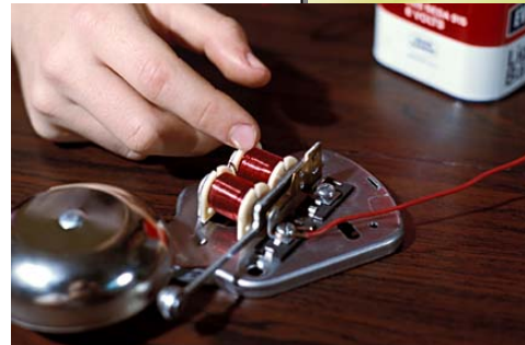
Electricity running through wire coils creates an electromagnet, like the kind found in doorbells, headphones, and other common devices.
